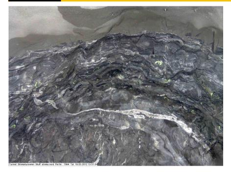
The high-resolution camera shows details in the geology pattern. The lighting is from the headlights of the vehicle the camera is mounted on.
