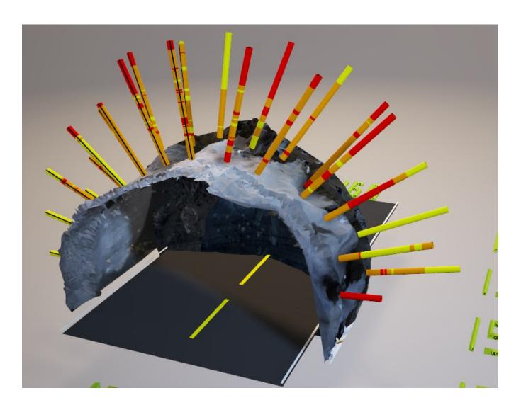
Documentation options are numerous when high-quality pictures are collected. Here, a 3D view with MWD-logged bolts, and camera pictures projected onto profiler scan (requires navigated camera system).
