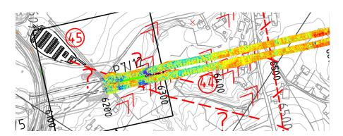
Interpreted hardness based on MWD data, superimposed
