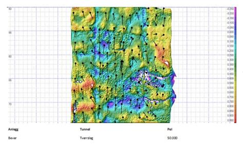
Flattened out map shows over- or underbreak, and bolt positions.
